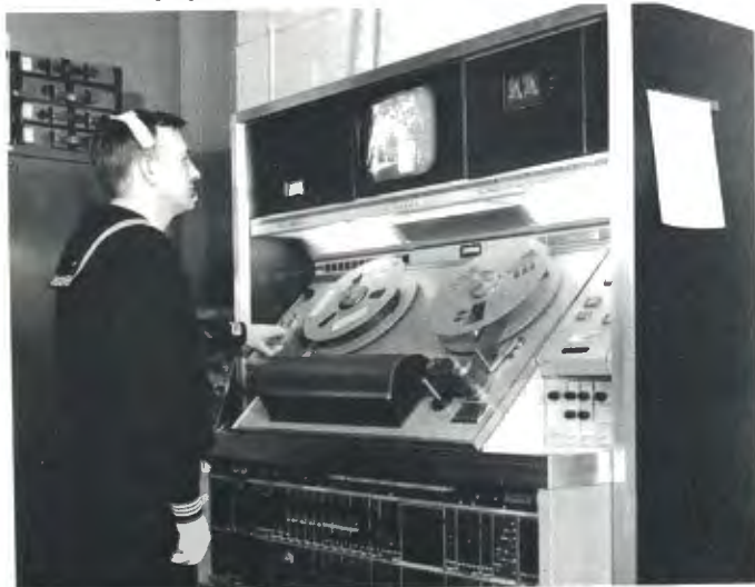
FIG. 4. Television tape machine used for recording TV studio pickups. Also used for playback of TV tape recordings to feed the Kine-Recorder.
