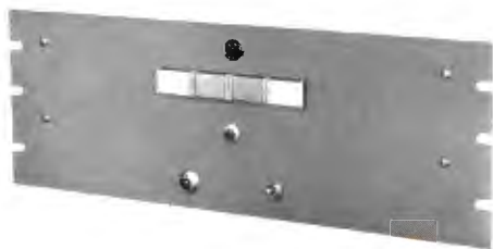
FIG. 4. The studio portion of the BTRA-5A Tone-Alarm System. This unit, in combination with the one shown below, constantly monitors five separate parameters at the transmitter site.
