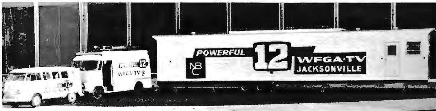
FIG. 26. Large mobile unit is converted house trailer 56-ft. long. It's especially designed for use at the Cape. It incorporates six cameras, tape and film systems, briefing room and news office.
