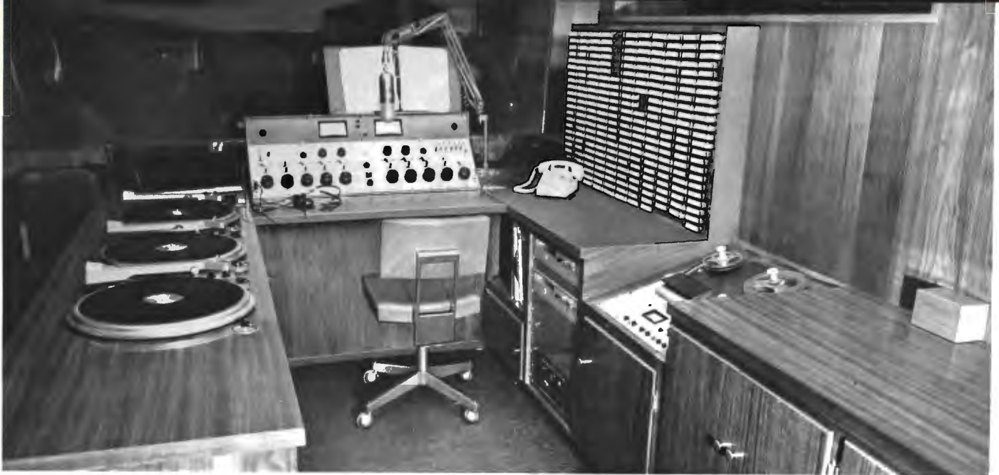
FIG. 4. Master Control is equipped with three turntables, a reel-to-reel tape deck, two cartridge-tape machines and, of course, the control console. Note cartridge-storage bins above cartridge-tape machines.
