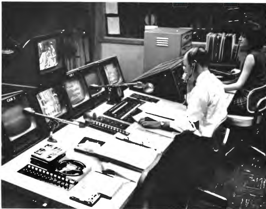
FIG. 17. Control Room "A" where all live productions are directed. Positions (L. to R.): producer, director, audio. In upper right is announce booth. Key switches on left of video switcher for inter-com to all production positions. RCA custom switcher panel is part of a TS-40 system.
