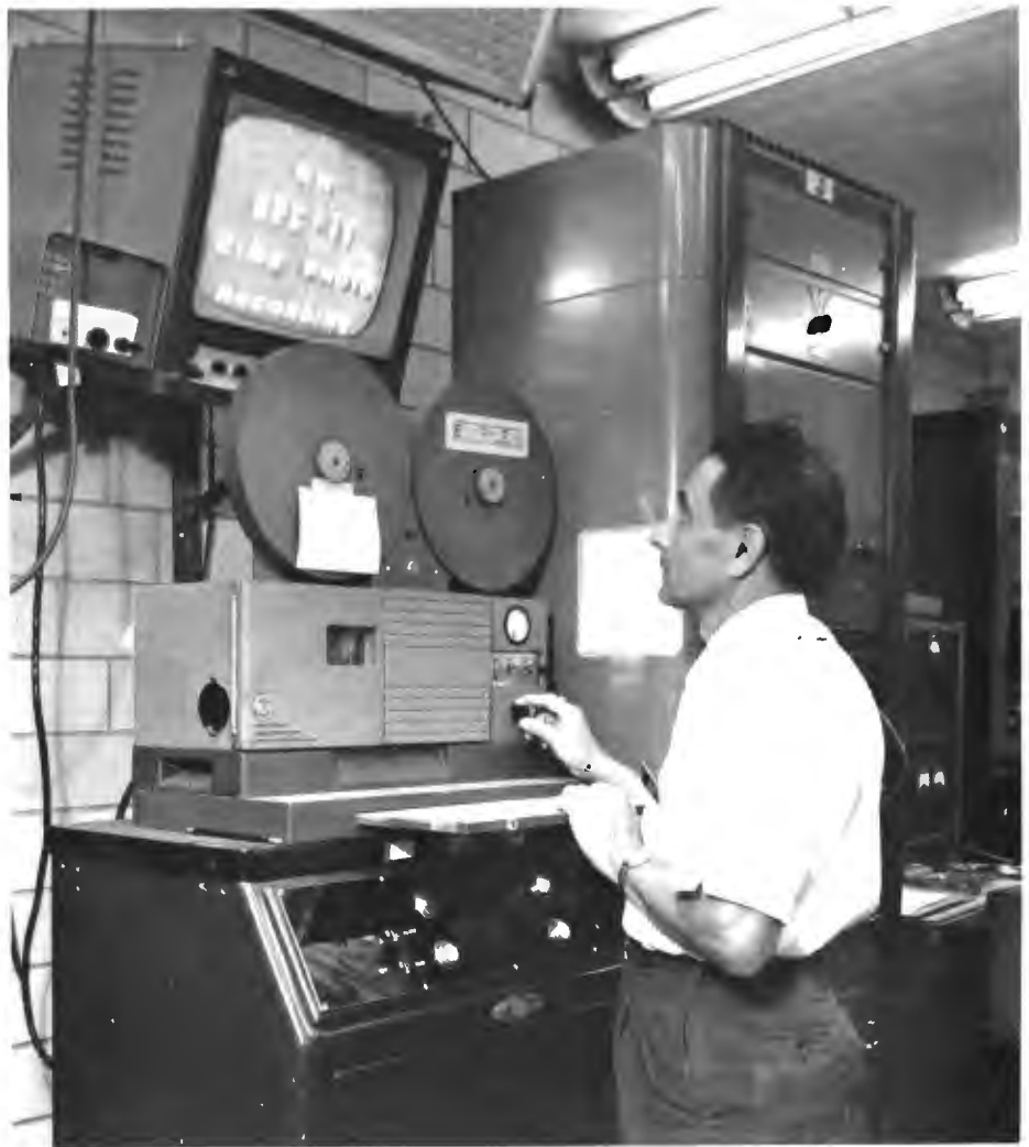
FIG. 18. RCA optical sound recorder used at NPC to record sound on film by using the double system.
