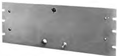
FIG. 5. The transmitter unit of the BTRA-5A Tone-Alarm System. This unit utilizes one of the remote-control telephone pairs to communicate with its studio counterpart.
