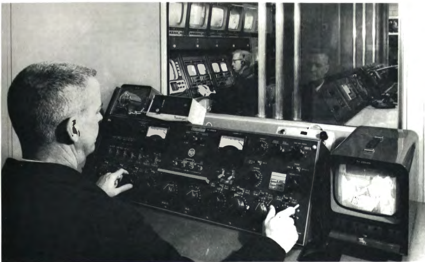
FIG. 13. Audio booth, showing BC-6 Dual Channel Console and TM-9 picture monitor. (Note that audio operator can see into control room.)
