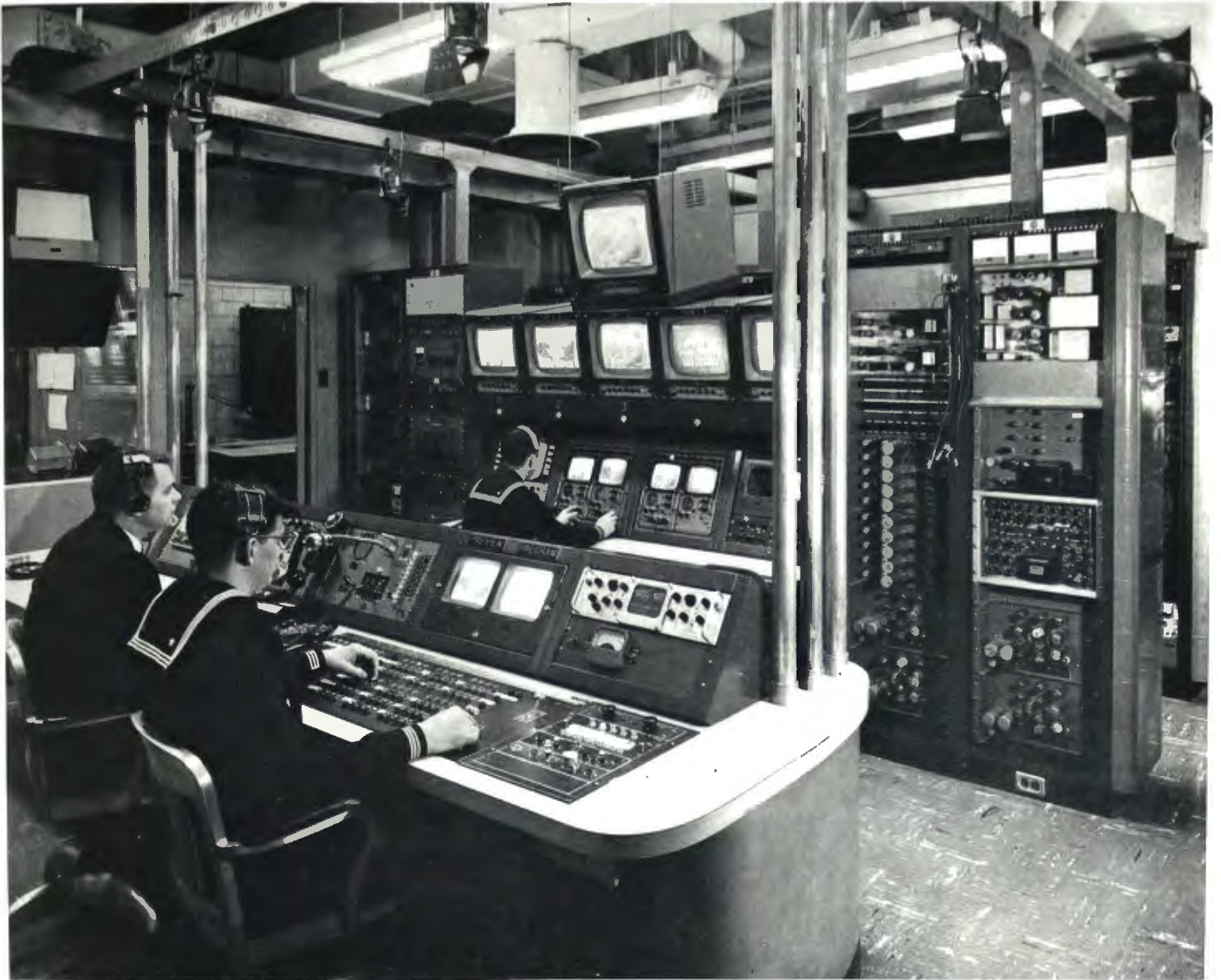
FIG. 21. TV control room at NPC. In foreground is switching and effects position, in rear, video control position (camera controls). Overhead monitors preview picture sources for program director and display on-air signal.
