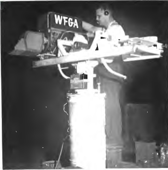
FIG. 27. TK-31 Camera assembled on machine gun mount for tracking to vertical position at the Cape.
