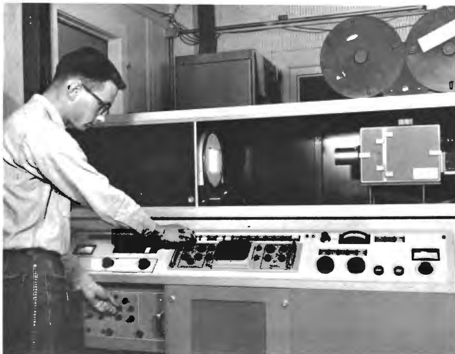
FIG. 16. Controls of Film Recorder are preset to desired standards. Automatic circuits maintain these standards throughout film recording.
