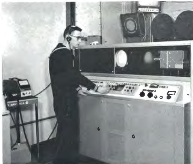
FIG. 5. RCA TV Film Recorder which transfers TV signals (from the TV Tape machine) to 16mm film stock (positive or negative.)
