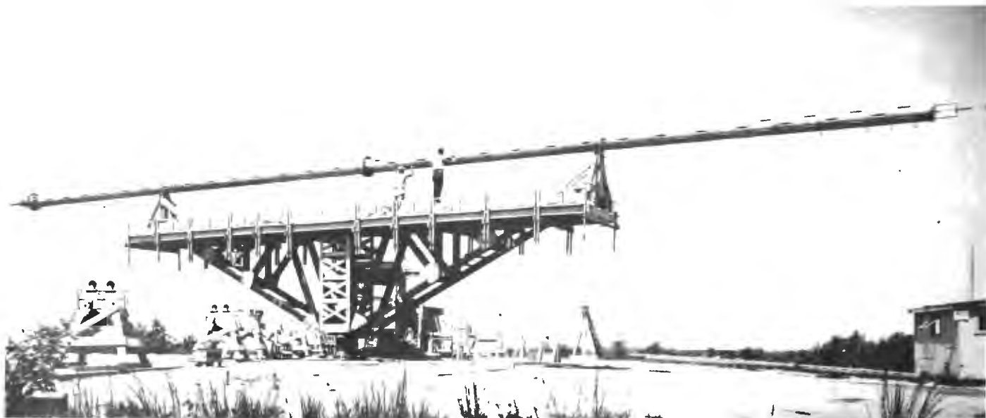
FIG. 10. The horizontal turntable at RCA's 40-acre antenna-test site in Gibbsboro (N.J.). This wooden, trestle-like device allows radial and axial rotation of the antenna under test so that measurement of the vertical radiation patterns can be made in any antenna plane. The antenna shown here is an RCA-Pylon device for UHF television transmission.
