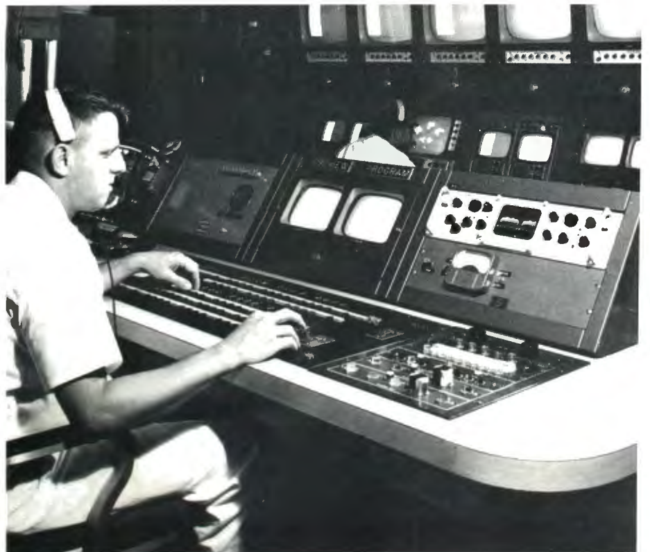
FIG. 10. Close-up of program switching position showing video switcher and remote control and switching panel at right.
